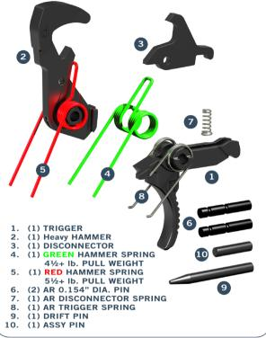
EDT® HG fire-control group (FCG) parts are shown in the figure by name and quantity.
