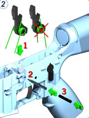
Choose the red spring for a  $5\frac{1}{2}$ + lb. trigger pull weight or the silver spring for  $4\frac{1}{2}$ + lbs. Install the hammer sub- assembly into the lower receiver just like you would a stock AR hammer, making sure the hammer spring's arms nest in the spaces on either side of the trigger in the lower receiver to retain the trigger pivot pin. Use the drift pin as desired.
