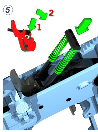
Inspect the fire-control for proper toggle spring installation and function whenever live-fire exercise is intended, especially if you had the fire-control installed by someone else, or if you loaned your rifle to someone else.
