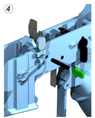
Complete installation of the hammer subassembly by inserting the stock AR 0.154-inch diameter pivot pin like you'd install a stock AR hammer.
