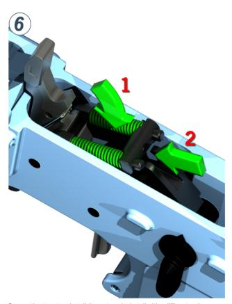
Reverse the steps to uninstall the parts and reinstall with a different spring combination to change trigger pull according to the table. Use a pointed tool inserted into the toggle pivot at the arrow for convenient removal and reinsertion.
