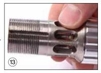
If the Case Trim Xpress is stored in a humid environment or for a length of time you can add a light coat of oil to the Adjuster Barrel and cutter head to prevent corrosion.
