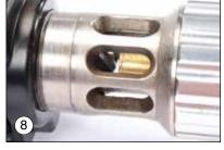
TRIMMING TIP: when setting the initial cutting depth make sure you have fully compressed the spring; repeat this step a few times, to ensure the proper initial setting.
