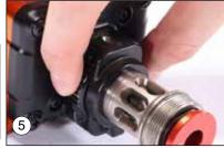
wise will INCREASE your cutting depth (more material removed). A viewing window is located at the top of the adjustment wheel housing, this window will allow the user to view the graduation marks to ensure a proper setting.
