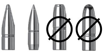
Bullet lengths from approximately .80" to 1.05" will use the short feed block. Bullet lengths from approximately 1.05" to 1.55" will use the tall feed block. Do not use bullets outside this range.
